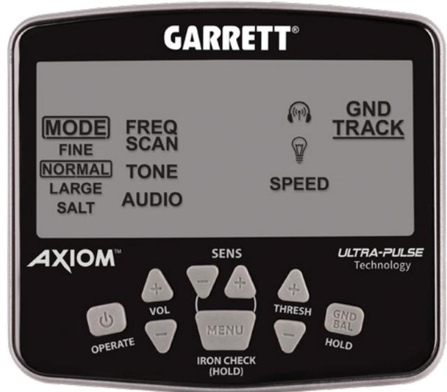
Press MENU to highlight MODE, then use Plus (+) or Minus (-) button to select the desired Mode. Only the selected Mode will remain on the LCD when the Menu is exited.
