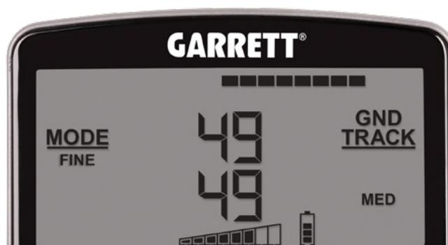
This detected target is causing the upper row of pixels to swing to the right, which corresponds with a target creating a high tone..
