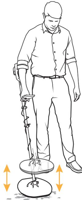
During a Ground Balance procedure, GND BAL will display on the LCD. Dual Ground Balance values are shown by the upper and lower 2-digit numbers.
