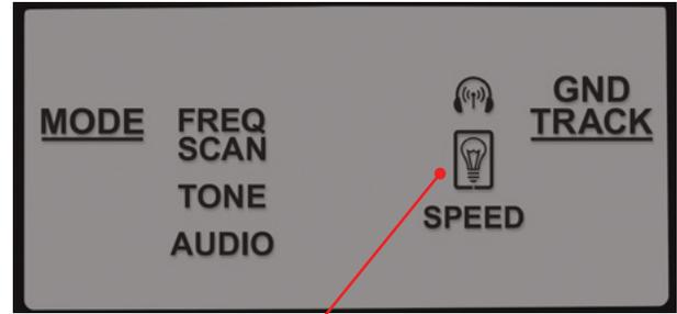
When Backlight icon is highlighted, use the Plus / Minus Menu buttons to switch on or off.
