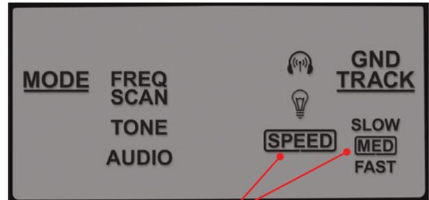
When SPEED icon is highlighted, use the Plus / Minus Menu buttons to select desired coil swing speed.
